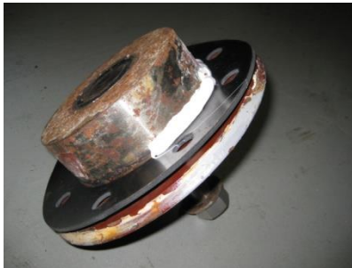
FIGURE 1 - 3M MARINE 5200 ADHESIVE ON ADAPTOR PLATE ON GASKET'S INSIDE EDGE
