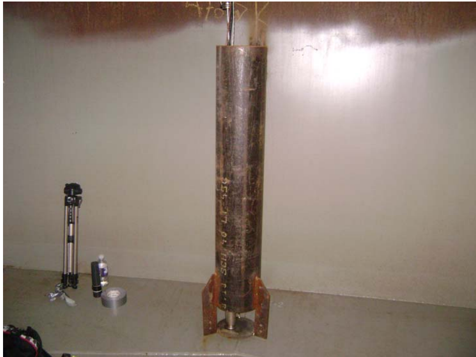
8" Gauge Tube with ITT Barton ATG Probe Assembly (Note: Gauge tube includes a datum plate approximately at chine elevation.)
