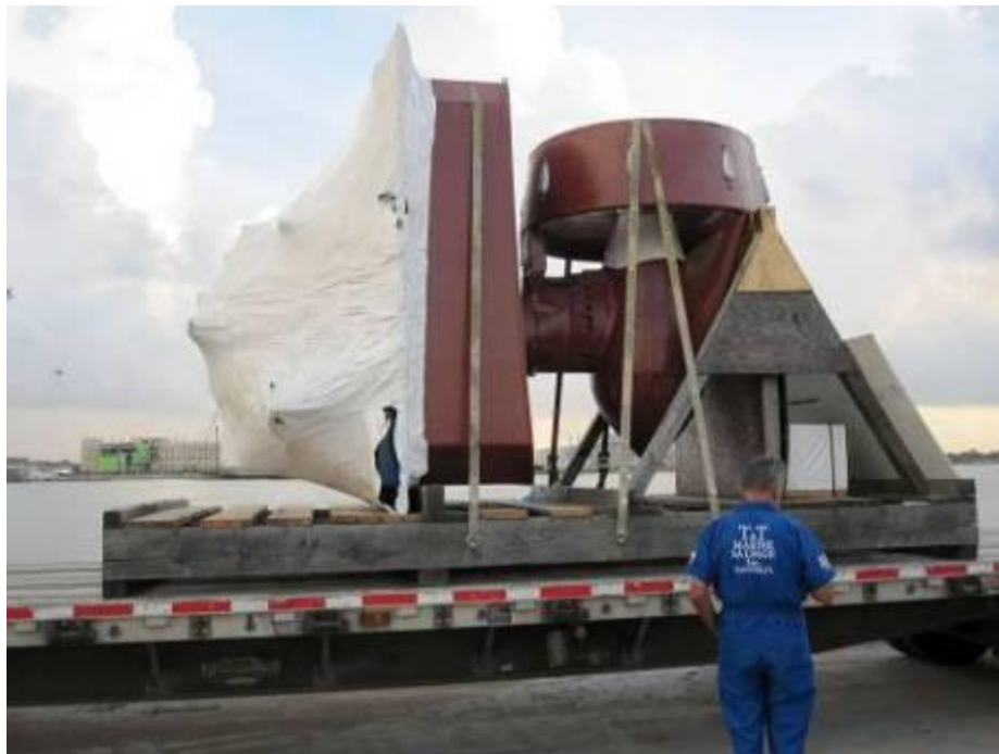
FIGURE 1. Z-DRIVE SHIPPING STAND AND SHIPPING ORIENTATION
