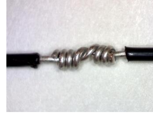
Figure 19-17. Completed Wrap for Western Union/Lineman Splice
