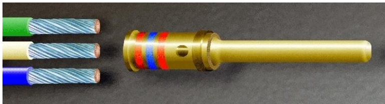
Figure 19-21. Stripped Wires Prior to Insertion
