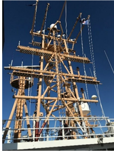
Pisces Antenna top main mast
