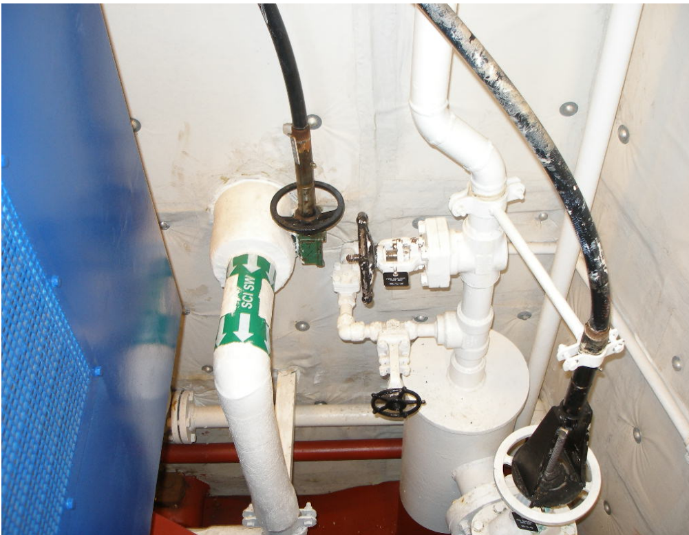
Fig. 3.8.1 Starboard side sea chest 2-inch vent and 3/4-inch air blow down valves; Port side sea chest similar
