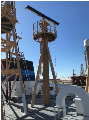
S-Band Radar Mast
