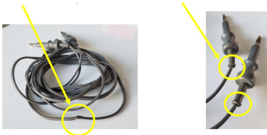
Figure 4—Cables/cords: examples of separation of the cord at the proximal end, nicks, lacerations, pin holes
