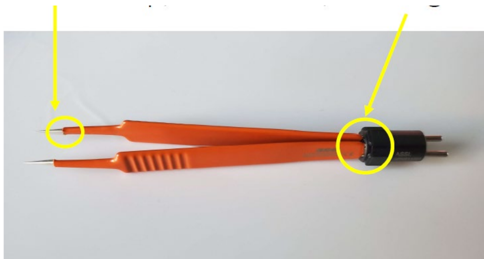
Figure 3—Insulated forceps: examples of frays at distal tip, lacerations, housing cracks
