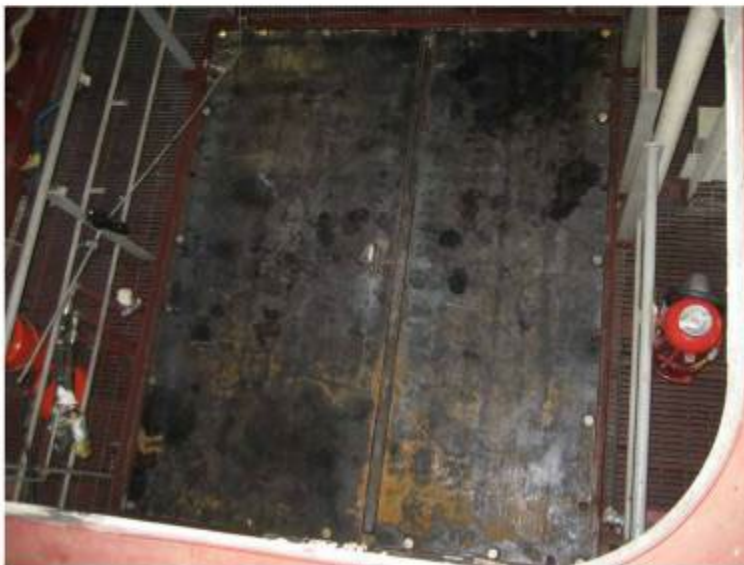
Figure, Z-drive Sea Well Covers Installed
