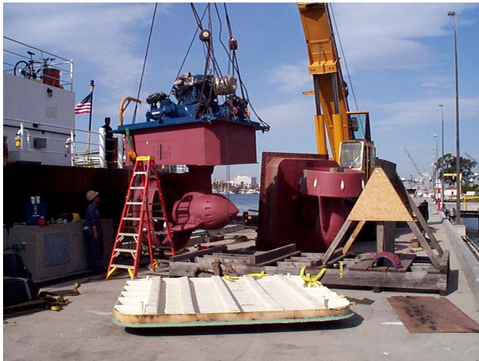
FIGURE 2. HISTORIC Z-DRIVE LIFTING ON-OFF CUTTER PHOTOGRAPH
