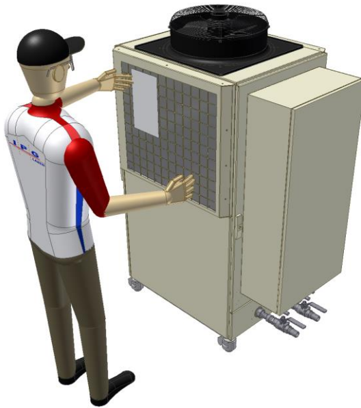
Checking rotation of the fan – sheet of paper must be sucked
