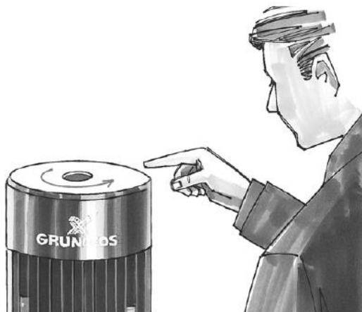
Checking rotation of the pump
