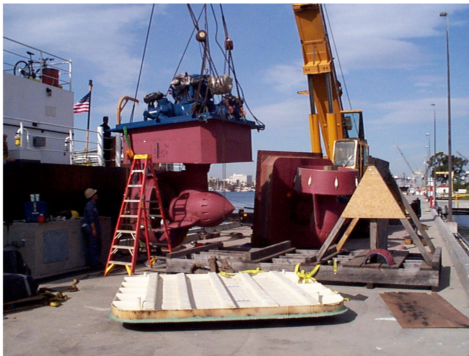
FIGURE 2. HISTORIC Z-DRIVE LIFTING ON-OFF CUTTER PHOTOGRAPH
