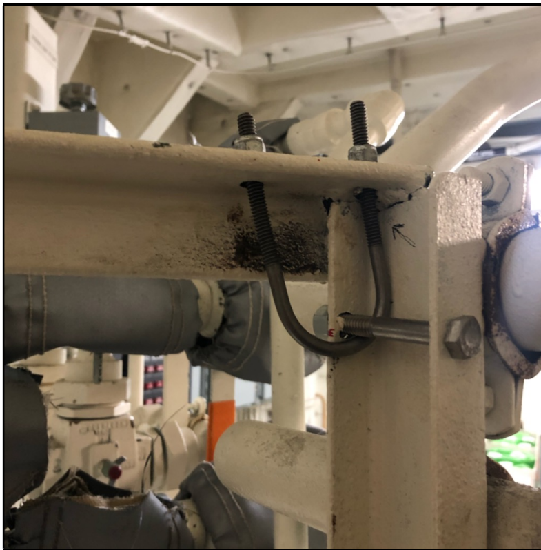
PHOTO 2 CRACKED STEERING HYD PIPE HANGER BRACKET DETAIL
