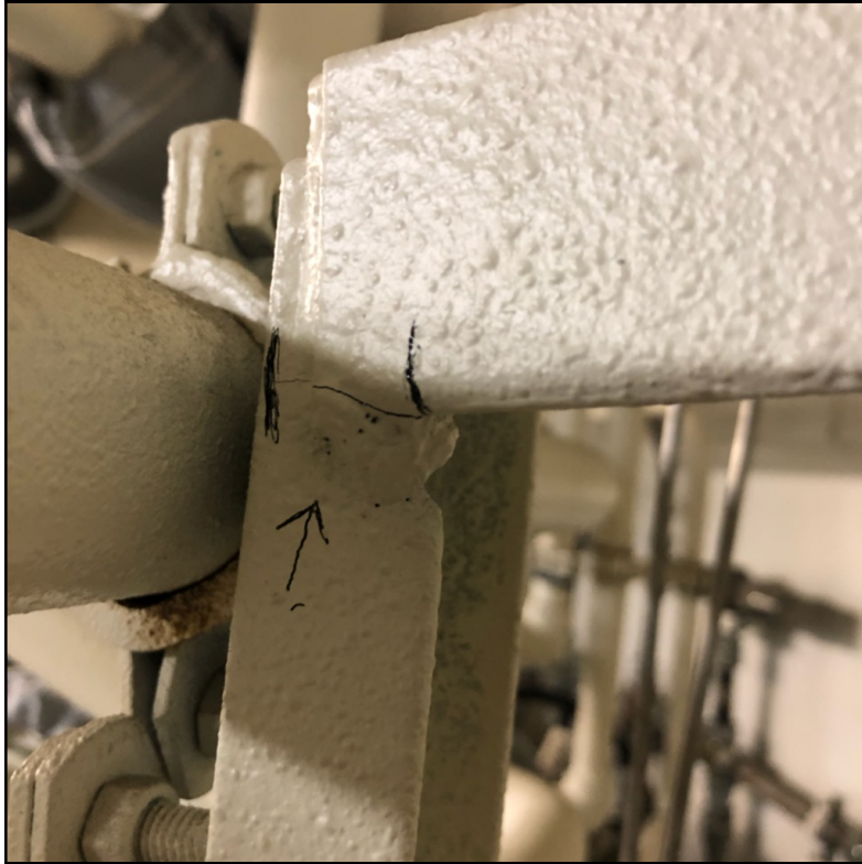
PHOTO 2 CRACKED STEERING HYD PIPE HANGER BRACKET DETAIL
