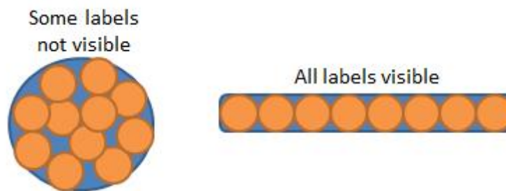
Figure 23: Cable Labels in Bundles
