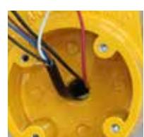
9. Strip the ends of the Blue and Brown leads and crimp a spade terminal onto each. If there are only two terminals, connect the Blue and Brown leads to the two pushbutton terminals in any order. Using the provided machine bolts, secure the pushbutton onto its frame.
