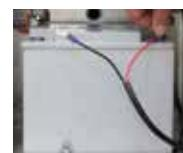
2. First, attach the ring terminal of the battery cable tagged 'Positive +' to the (+) terminal on battery. Secure with washer and nut.
