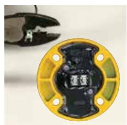
Note: If you use an alternative pushbutton with three terminals, connect the Blue lead to the pushbutton's 'COM' terminal and the Brown lead to the 'NO' terminal. Do NOT use the 'NC' terminal.
