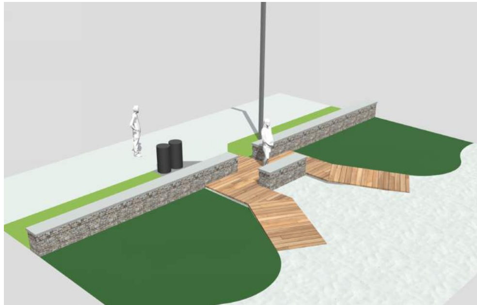
11 Sea Wall – gabion with concrete cap and wood decking
